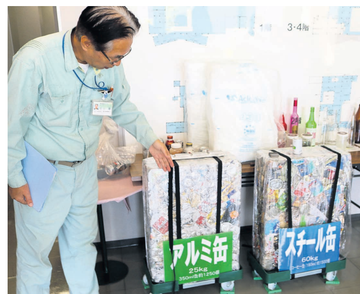
Minoru Nakagawa of the Resources and Waste Cycling Bureau explains that, even though they are the same size, the green-labelled bale of compressed aluminium cans weighs 25 kilogrammes compared to the bale of compressed steel cans weighing 60 kilogrammes.
